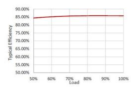
OT FIT 36 220-240 24 PC Typical Efficiency vs. Load
